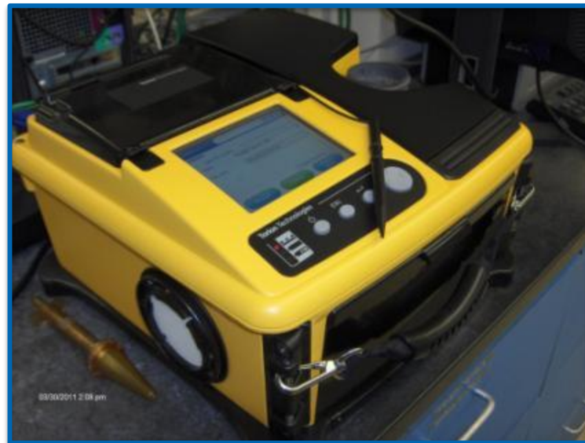
Portable GC-MS 31 lbs 50 sample battery life
